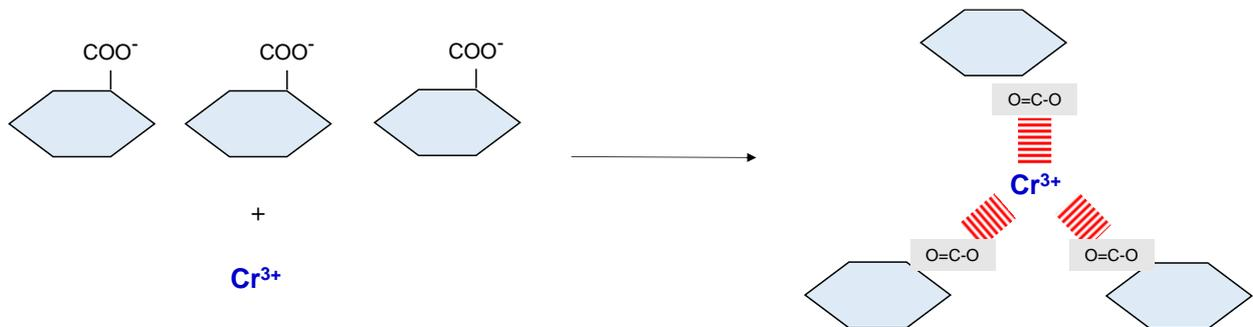
Figure. 2 Crosslinking of xanthan gum and  $\text{Cr}^{3+}$  ion
