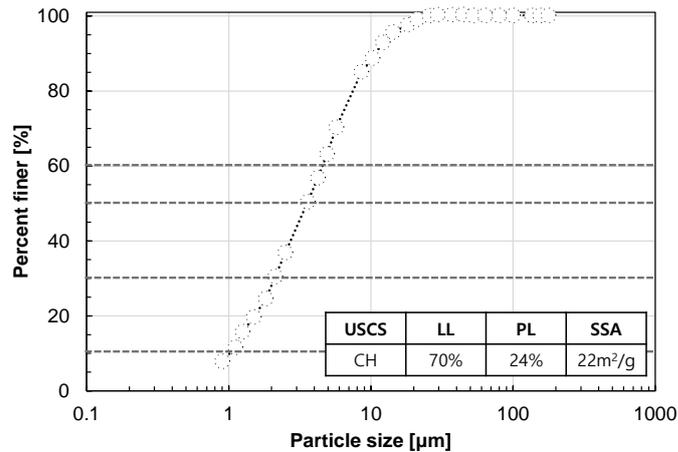
Fig. 1 Particle size distribution of Bintang Kaolinite
